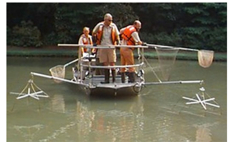
Right: electrofishing from a boat; an electric current stuns fish then they are caught in a net
